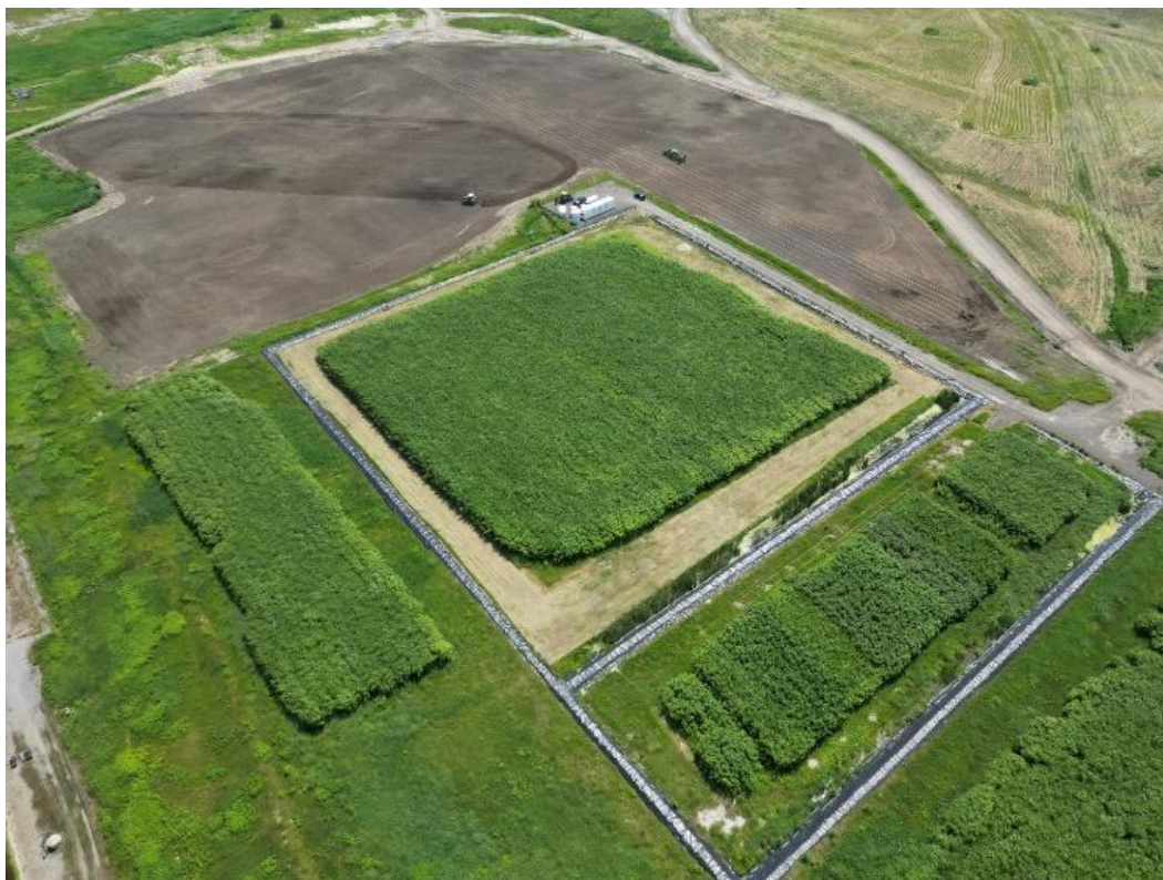
Figure 2. Example of 1.2-ha Evaplant system built by Ramo in 2018 on a Quebec landfill site (picture taken in 2023).
